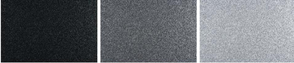
Figure 2.2: Images of same car paint with different exposure setting. From left to right:  $-2$  EV,  $0$  EV,  $2$  EV
