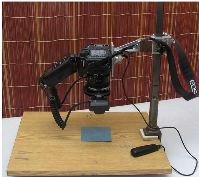
Figure 2.1: Camera configuration: Canon 30D, Canon EF-S 60mm Macro USM lens, Canon Macro Twin Lite MT-24EX flash and remote switch.
