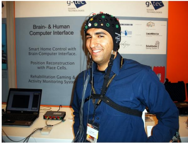
Figure 1.3: For a simple EEG session we need an electrode cap, a signal amplifier, a processing unit (the computer) and a feedback device (in this case a computer screen).
