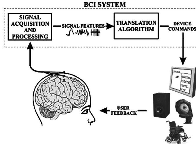
Figure 1.2: A BCI system diagram showing closed-loop paradigm. From [McFarland et al., 2006]
