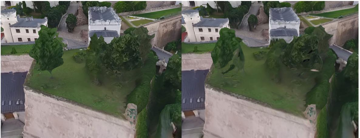
Figure 4.3: Featureless spot with trees. On the left is the ground truth model and on the right the reconstructed model.
