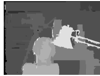
Figure 2: Tsukuba disparity map, modified dynamic programming on a tree
