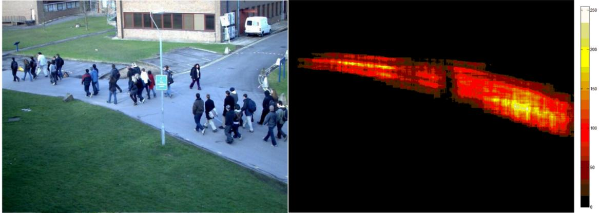
Figure 2.3: Constructed flow map of the scene model by multiview face detector, Xing, et al. [2]
