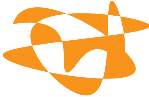
Figure 3.7: A shape filled using the even-odd rule.
