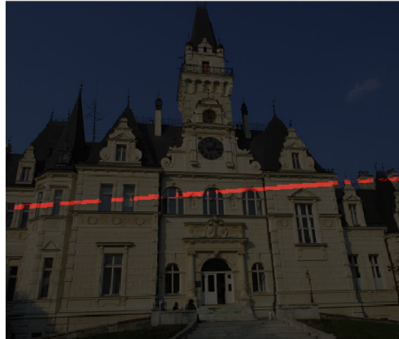
Figure 4.2: Probability map is reduced to red area after the epipolar line was computed.
