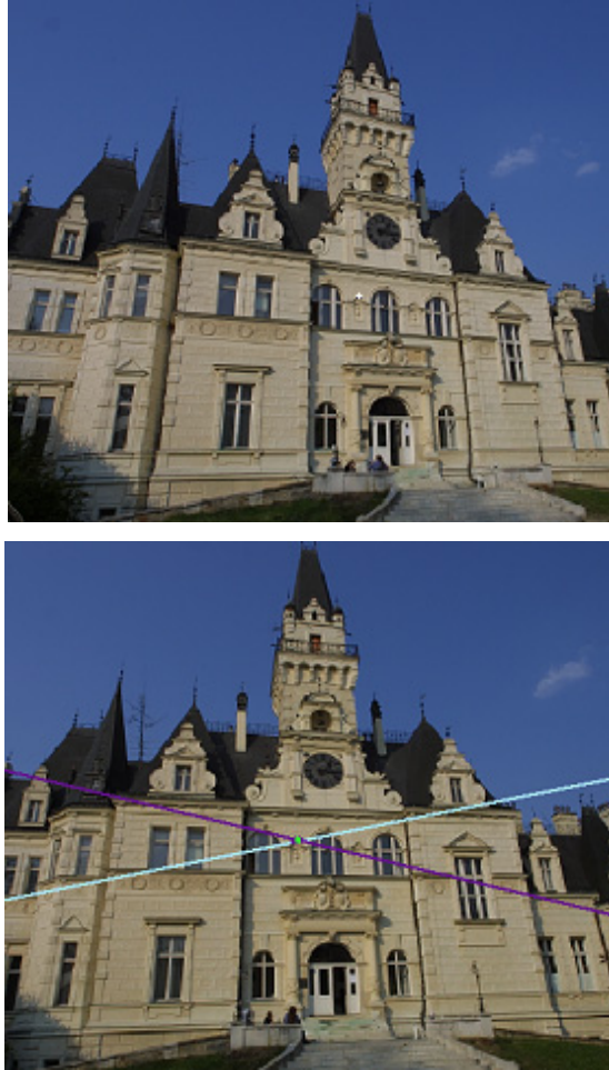
Figure 2.1: A light line is the epipolar line and a dark one is the false epipolar line. The corresponding point is located near their intersection.
