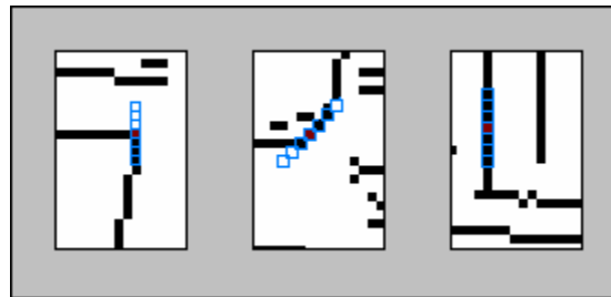
Figure 3.3: Masks for corner, curved edge and narrow edge are displayed.
