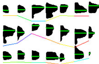
Figure 15: Detail of chunks. Green horizontal lines through chunks are places where maximums were found.
